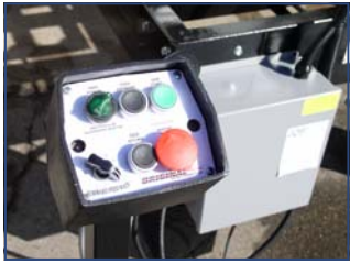
Photo at left shows the stand mounted control panel and electrics enclosure for optional powered carriage feed sys-
