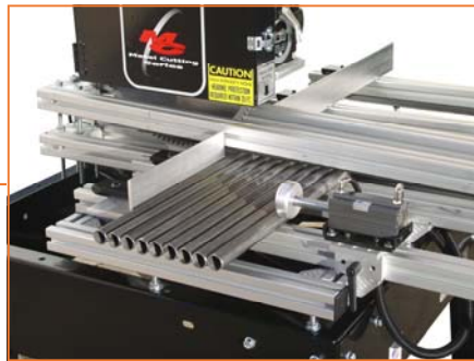
Above photos from right: rear pushing cylinder, (clamps material against fence) over arm clamping system (holds multiple pieces) over center clamp (presses material against t-slot extrusion) table
