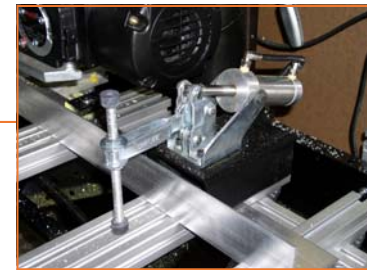
Above photos from right: rear pushing cylinder, (clamps material against fence) over arm clamping system (holds multiple pieces) over center clamp (presses material against t-slot extrusion) table
