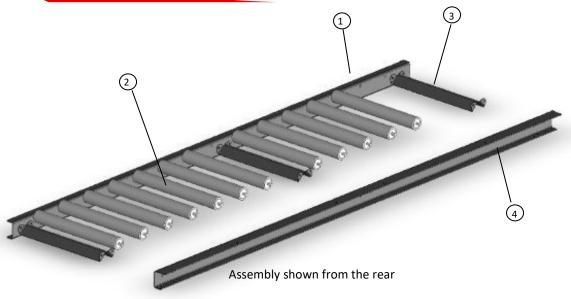
8' Roller Table Extension parts breakdown and
