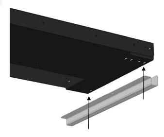
To attach the mounting bracket (after it has been bolted to the frame of the prospective machine) use the included  $5/16-18 \times .75$ " carriage bolts (2), flat washers (2), and hex nuts (2) to attach the mounting bracket to the brace (index # 2) that has been attached to the extension table (note bracket appearance will vary by model of machine / machine stand to which it is being mounted.
