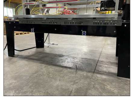
Mounting Brackets attached to a Beam Saw.
