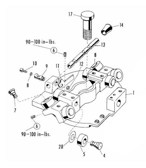
Item #2 and #3 are not used in 3579 Metal Cutter or 40005 Power Crossfeed
