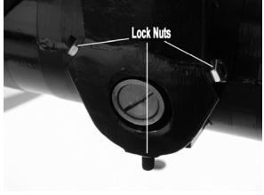
If after making these adjustments the blade continues to heel, particularly if the blade heels on both sides of the material, the blade may require tensioning. If the blade must be re-tensioned contact your local distributor.
