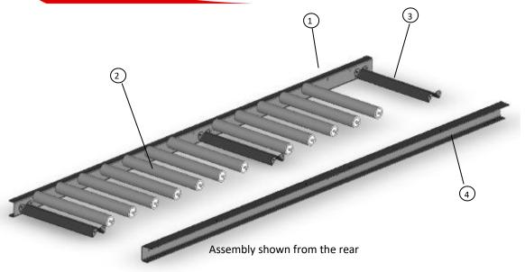
8' Roller Table Extension parts breakdown and
