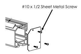
After the measuring system is installed and lined up, install the end plates, these plates will improve the looks of the assembly and keep sawdust out of the extrusion. To install simply line up the holes in the plate with the holes on the rails and attach using the 3 provided screws.
