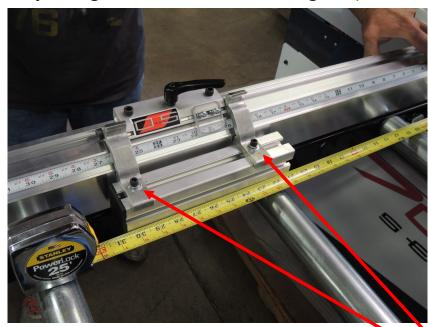
To move the front extrusion simply loosen the socket head cap screws, (Item#1) (about 1/4—1/2 turn) and slide the extrusion., then tighten the screws once the rail is set correctly.
