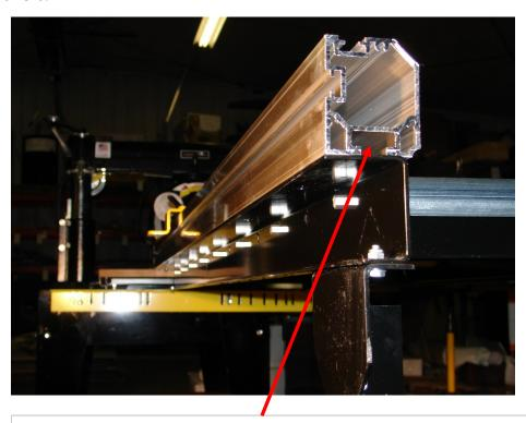
Square flat nut will insert in this T-slot on the bottom of the extrusion 3 flat nuts and 3 socket head cap screws and washers. This hardware will attach through the slotted holes in the rear (wider) flange on the tables.
