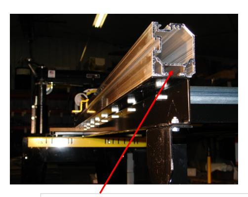
Square flat nut will insert in this T-slot on the bottom of the extrusion 3 flat nuts and 3 socket head cap screws and washers. This hardware will attach through the slotted holes in the rear (wider) flange on the tables
