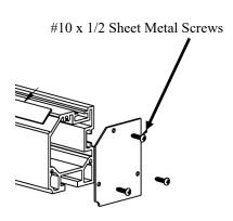
After the measuring system is installed and lined up, install the end plates, these plates will act as a stop on the outside end to keep the slider carriage from sliding off the end of the rail and will improve the looks of the assembly and keep sawdust out of the extrusion. To install simply line up the holes in the plate with the holes on the rails and attach using the 3 provided screws.
