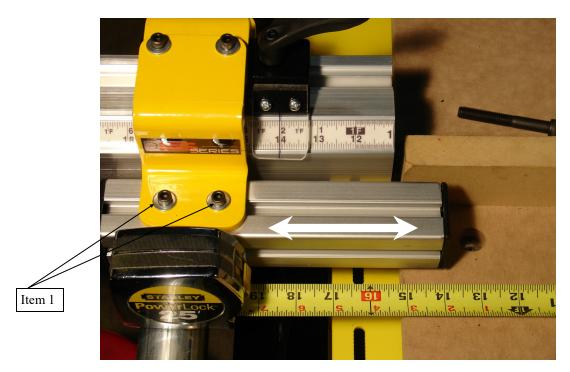
To set the clearance between the stop and the blade simply set a tape measure against the blade and set the stop at 14" on the back stop tape. Then adjust the front extrusion to the 14" mark on the tape measure. To move the front extrusion simply loosen the socket head cap screws, (Item#1) (about 1/4—1/2 turn) and slide the extrusion., then tighten the screws once the rail is set correctly
