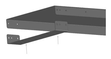
To attach the mounting bracket (after it has been bolted to the frame of the prospective machine) use the included  $5/16-18 \times .75$ " carriage bolts (2), flat washers (2), and hex nuts (2) to attach the mounting bracket to the brace (index # 2) that has been attached to the extension table (note bracket appearance will vary by model of machine / machine stand to which it is being mounted.
