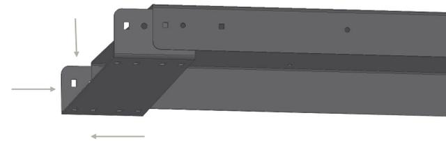
To attach the mounting bracket (after it has been bolted to the frame of the prospective machine) use the included 5/16 –18 x .75" carriage bolts (2), flat washers (2), and hex nuts (2) to attach the mounting bracket to the brace (index # 2) that has been attached to the extension table (note bracket appearance will vary by model of machine / machine stand to which it is being mounted).
