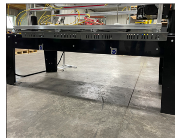
Mounting Brackets attached to a Beam Saw.
