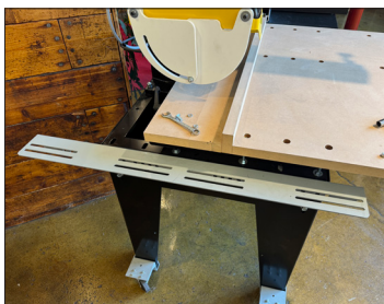
Mounting Bracket attached to a Contractor Duty Radial Arm Saw.
