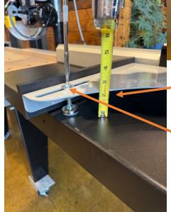
Using a tape measure height off the table at the fence and match that height out on the end using the foot and a screwdriver. Once level lock the stud using the jam nut.
