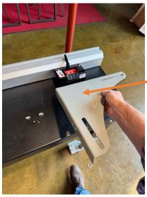
Rotate gang stop bracket depending on which way the stop will be mounted.
