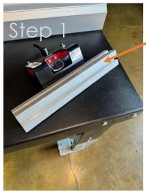
Remove the aluminum foot from your fixed foot slider assembly. Once removed you're system should look like the photo at the right
