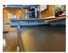
Attach the HDPE foot on the front side of the bracket using these holes and running the socket head cap screws in from the front side as shown with the hex nuts on the inside. Note use the further outside holes. Using these holes will allow adjustment on the front side in the next step.
