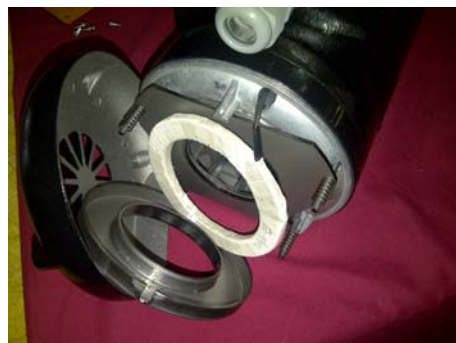
View showing the fan cover and coil pulled from the coil housing. Note the location of brake springs on the tie rods.
