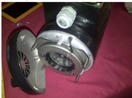
View showing fan cover removed. Note the coil housing sitting in the mounting tabs from the fan baffle casting.
