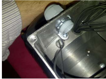
View showing the access hole where the coil wires pass into motor box. Note the hole where the leads protrude. Be careful to not drop any parts down these areas.
