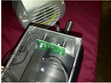
View showing the brake module mounting and plugged in coil wires.
