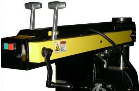
Manual Chain Carriage Feed Standard on 22" machines
