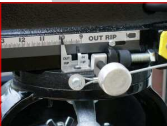
Rip Lock knob, 'in rip' & 'out rip' pointers
